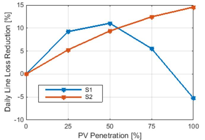
Fig. 6. Daily line loss reduction of the two investigated configurations at different PV penetration levels in comparison to the base case of 0% PV penetration.
