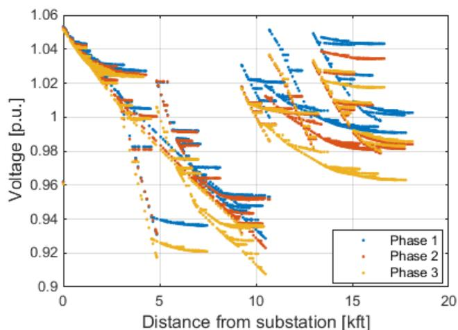
Fig. 1. Voltage profile from OpenDSS simulation along the investigated feeder at max load demand when solar resource is not present.
