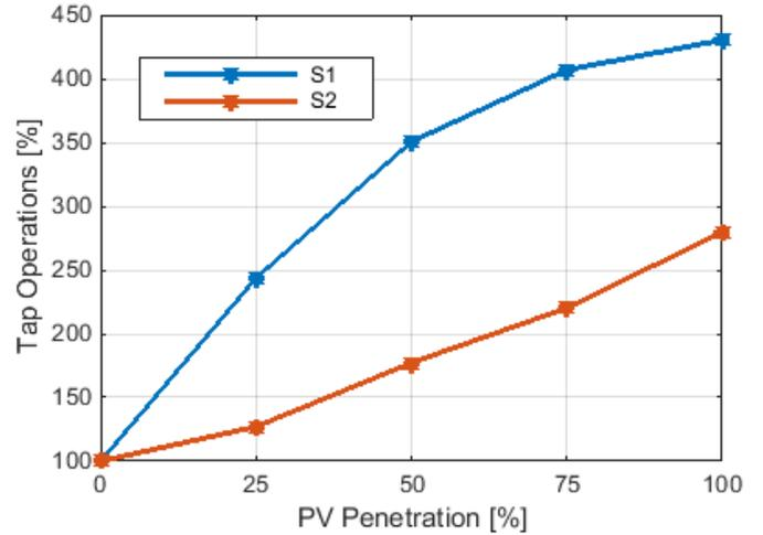
Fig. 5. The percentage change in number of tap operations of the two investigated configurations at different PV penetration levels in comparison to the base case of 0% PV penetration.
