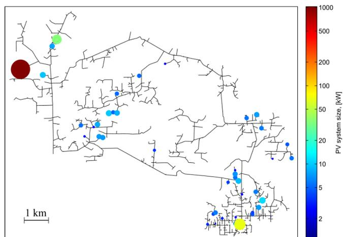
Fig. 2. Topology of the investigated feeder with 11MW load and 2.3MW PV. This is used as centralized configuration.
