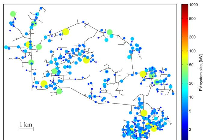
Fig. 3. The distributed configuration of the investigated feeder with 430 small PV systems.
