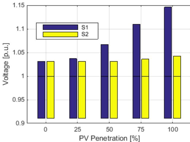
Fig. 4. Voltage range at different PV penetration levels of the centralized (S1) and distributed (S2) configurations.
