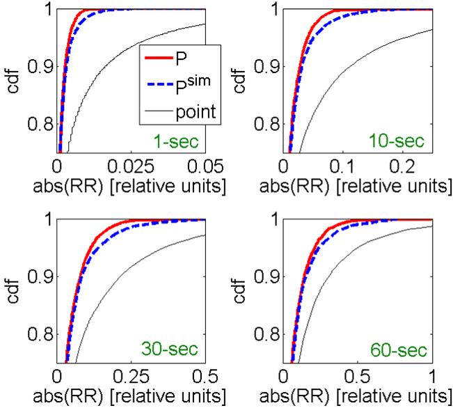
Fig 9. Comparison of extreme (>75<sup>th</sup> percentile) RR distributions at Ota City on July 16<sup>th</sup>, 2007 for the actual power output (red solid line), WVM simulated power output (blue dashed line), and a point sensor (black thin line) at 1-sec (top left), 10-sec (top right), 30-sec (bottom left), and 60-sec (bottom right) timescales. Units on the x-axis were multiplied by an arbitrary scaling factor to be consistent with Fig 10.
