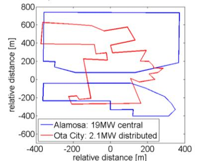
Fig 1. Footprints of the Ota City and Alamosa PV plants showing their areas relative to one another. The Ota City plant covers  $0.278\text{ km}^2$  and the Alamosa plant covers  $0.623\text{ km}^2$ , giving PV densities of  $7.55\text{ W m}^{-2}$  (Ota City) and  $30.5\text{ W m}^{-2}$  (Alamosa).
