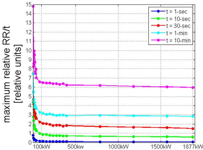
Fig 3. Maximum RRs at various timescales on July 16<sup>th</sup>, 2007 at Ota City. The points represent various combinations of houses: from 1 (~4W) to 477 houses (1877kW). Values on the y-axis were multiplied by an arbitrary scaling factor for consistency with results from Alamosa (Fig 4).
