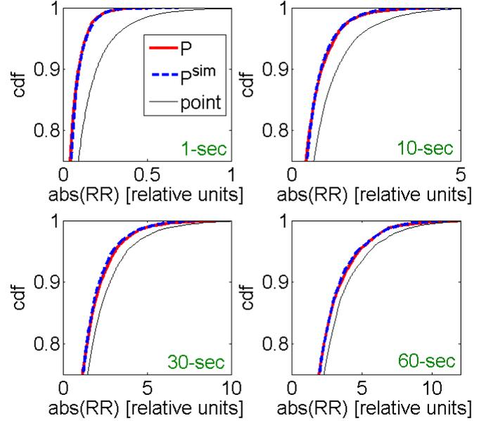
Fig 10. Comparison of extreme (>75<sup>th</sup> percentile) RR distributions at Alamosa on February 11<sup>th</sup>, 2012 for the actual power output (red solid line), WVM simulated power output (blue dashed line), and point sensor (black thin line) at 1-sec (top left), 10-sec (top right), 30-sec (bottom left), and 60-sec (bottom right) timescales. Units on the x-axis were multiplied by an arbitrary scaling factor to protect the confidentiality of the power data.
