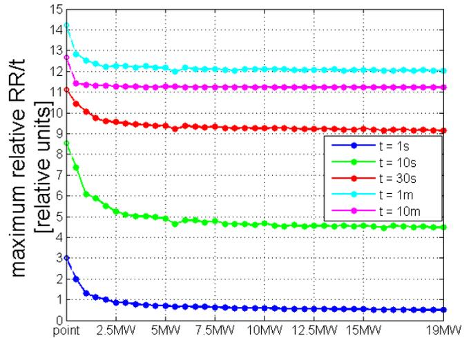
Fig 4. Maximum RRs at various timescales on February 11<sup>th</sup>, 2012 at Alamosa. The far left hollow point is the point sensor, while the solid points are 1 (0.5MW) to 38 inverters (19MW). Values on the y-axis were multiplied by an arbitrary scaling factor to protect the confidentiality of the power data.
