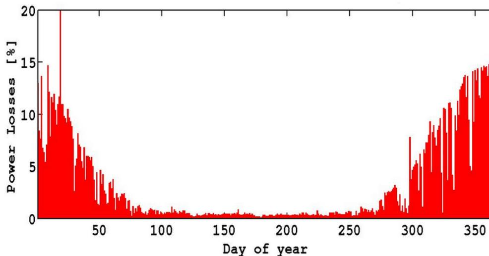
Figure 3. Estimated losses due to horizon obstruction of the sun for the year 2011. They are calculated as a percentage of the daily power production that would be lost if compared to a obstructions free horizon.
