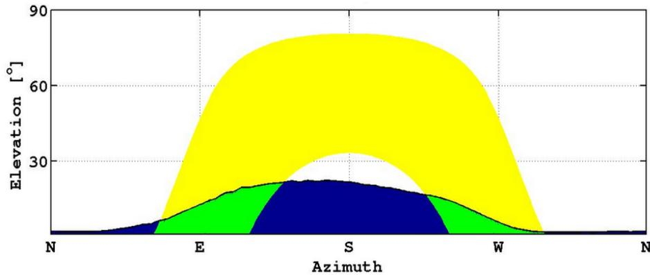
Figure 1. Horizon (blue) and sun trajectories along the year (yellow). The portions where the elevation is shading the direct sunlight are painted in green.
