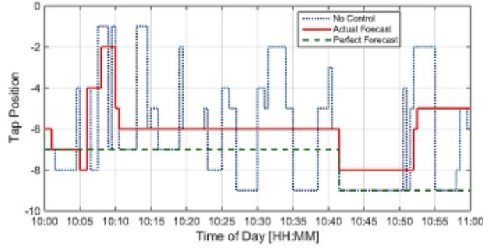
Fig. 1. Tap position sequences of transformer 3 at 10am-1pm on Jan 19, 2015 for three different scenarios. Originally the number of TO was 135. Using the actual and perfect forecast that is reduced to 17 and 2, respectively.
